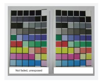
Figure 5 - Simulated 40-Year Indoor Light Fade Test: Just Printed (left) vs. Print Subjected to Fade Conditions
