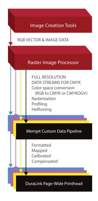
Figure 2 - DuraLink Data Pipeline with Dot-Level Control
