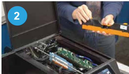
2 Do not touch any part of the electrical contacts or ink ducts.
