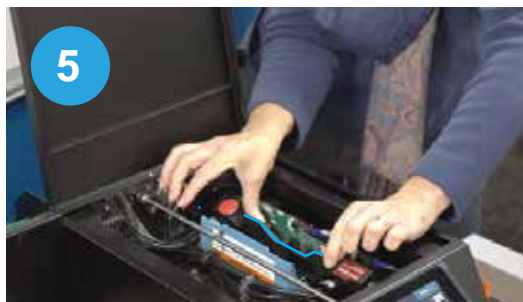
5 Place in at 45° angle and push back. Make sure it locks into place. You will hear a “click.”
