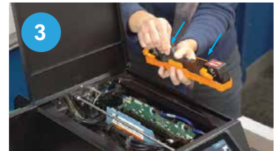
3 Take printhead out of orange cap and hold on handles for next step.
